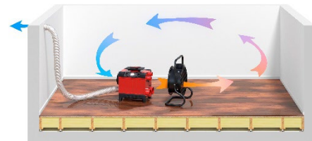
The wet air must always be evacuated via hose out from the space to be dried. The image shows room drying.
