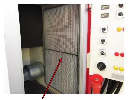
Make sure to change filter at regular intervals depending on where the dryer operates. This is process air filter. (Art no. 05111).
