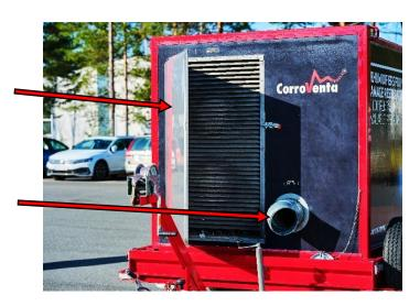
Control panel located on side door. Air hoses together with power cables are stored in this compartment.
