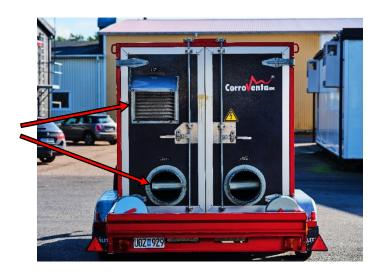
Open hatch for process air and remove sleeve for wet air.
