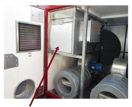
Make sure to change filter at regular intervals depending on where the dryer operates. This is the reg air filter. (Art no. 05110).
