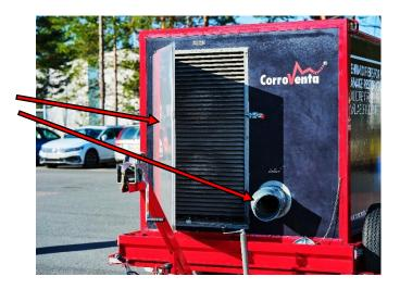
Connect dryer to 400V 63A with 63A cable.
